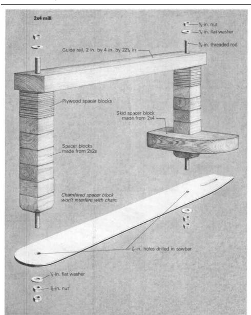
An accurate and inexpensive mill can be built from a dressed 2x4, two feet of  $\frac{1}{2}$ -in. threaded rod, four  $\frac{1}{2}$ -in. flat washers, six  $\frac{1}{2}$ -in. nuts, and a few scraps of 2x2s and plywood for spacers. Use several thicknesses of plywood, such as  $\frac{1}{4}$  in.,  $\frac{3}{8}$  in.,  $\frac{1}{2}$  in.,  $\frac{5}{8}$  in. and  $\frac{3}{4}$  in., so you can set the cutting height accurately.
